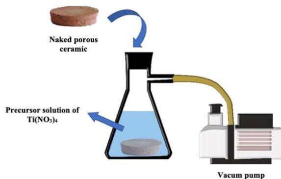
**Figure 1** The illustration of impregnation process at vacuum condition
