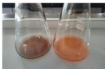
Figure 3 Before (a) and after (b) end of titration for standardization HCl with extract indicator
